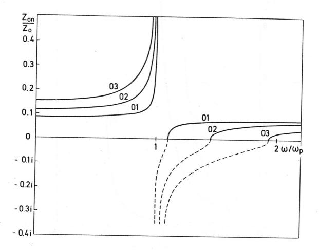
Fig.3 Characteristic wave impedance for radial modes in zylindrical plasma wave guide at infinite magnetic field.
