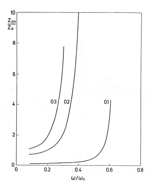
Fig.2 Characteristic mode impedance for radial modes in units of free-space impedance  $Z_o$ .
