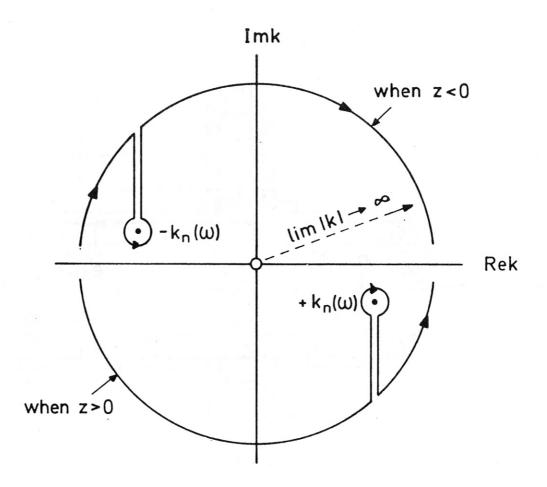
Fig.5 Complex wavenumber plane with displaced contours of integration used in residue calculation of Eq.(14.1)
