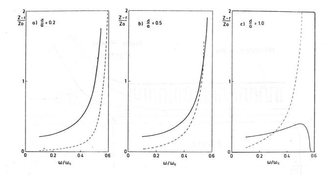
Fig.6 Gap-input impedance due to first three radial modes in zylindrical plasma waveguide, in units of free-space impedance, Z<sub>o</sub> = 377 Ohm.
