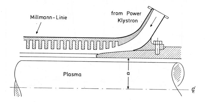
Fig.7 Sketch of proposed slow-wave directional coupler
