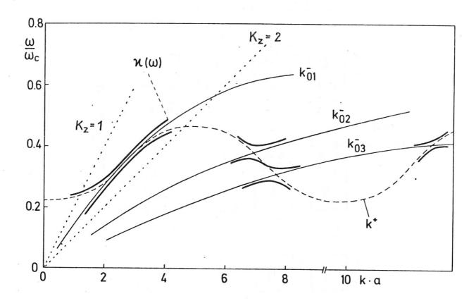
Fig.ll Dispersion characteristics of slow wave directional coupler to radial modes in a cylindrical plasma waveguide
