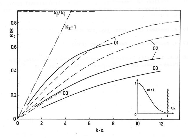
Fig.1 Electromagnetic wave dispersion in cylindircal waveguide filled with cold magneto plasma
