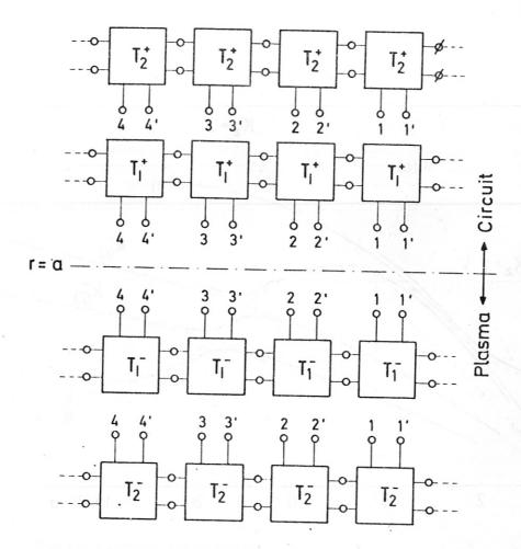
Fig.lo Chains of mode-equivalent T-junctions connected in parallel at the gap input terminals p p
