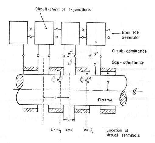
Fig.8 Coaxial model of slow-wave directional coupler.
